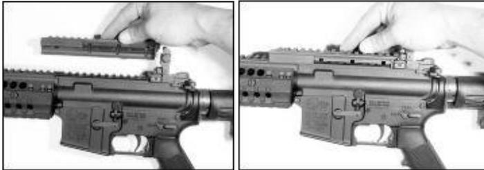
**Step 2 :** With the top rail in position insert the three square rods through the cross notches until the side bar engages the receiver. Secure the side bar to the receiver from the opposite side using the three provided nuts and tighten.
